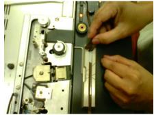
Figure 5 Slicing tape replacing
